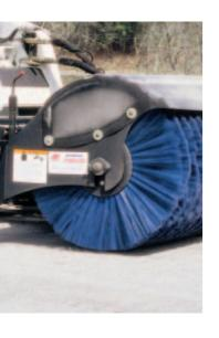
A quick-tach water kit is available for the S130 and all larger loaders to help control dust when using sweeping and angle brooms. (Kit purchased separately.) Operator controls downforce. Tilting the broom forward increases downforce to remove dried mud; tilting the broom back reduces downforce to extend bristle life.
